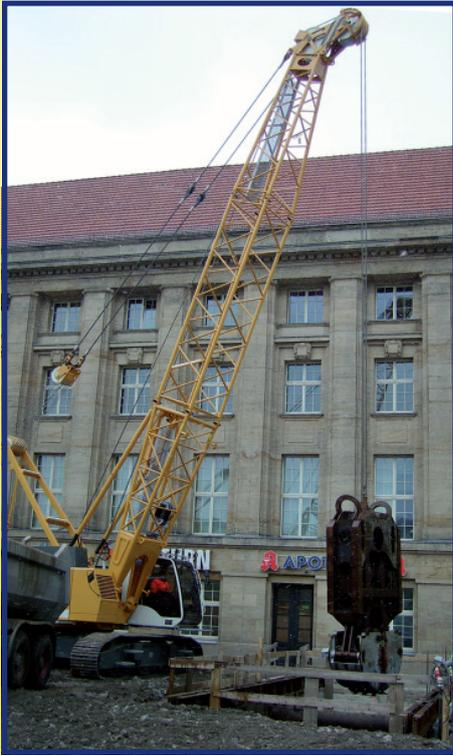
The cutting edges of the grab jaws are made of Hardox steel 450 and were especially hardened. Easy mounting of the grab jaws for excavation widths 800/1000/1200/1500 mm. All the grab teeth as well as all the wire rope pulleys are quickly exchangeable due to their construction as ready to use components.
