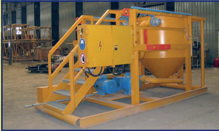
Batching plant for the mixing of liquid and powdery components. The equipment consists of a mixing tank including a mixing scale, an electrical mixing pump, several control valves and connecting piping. The fresh water inlet and the suspension outlet are marked as 4" fast clutch connections. Optionally it is also possible to mount "Storz" connectors. The feed of the powder can be achieved by using single bags or by using a scale and a screw-conveyor.
