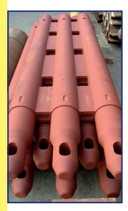
A flat stop end element consists of a welded construction comprising three parallel tube segments, each with a socket and tappet, several lining plates and, if required, additional extensions. A complete strand is formed by the assembly of individual stop end elements and normally incorporates a reinforced head piece, a bottom element and several intermediate elements. It is possible to adapt the extensions according to the excavation width.
