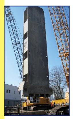
The cutting edges of the chisel are made of Hardox steel 450 and when required should be hard faced with 600 HB. All chisel types can be delivered with diverse hitching attachments and diverse cleaning devices
