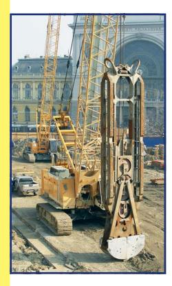
The cutting edges of the grab jaws are made of Hardox steel 450 and were especially hardened. Easy mounting of the grab jaws for excavation widths 800/1000/1200 mm. All the grab teeth as well as all the wire rope pulleys are quickly exchangeable due to their construction as ready to use components.
