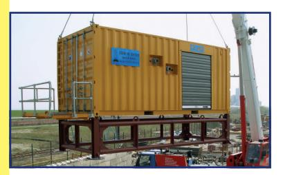
Batching plant for the mixing of liquid and powdery components. The equipment consists of a mixing tank including a mixing scale, an electrical mixing pump, several control valves and connecting piping. The fresh water inlet and the suspension outlet are marked as 4" fast clutch connections. Optionally it is also possible to mount "Storz" connectors. The feed of the powder can be achieved by using a scale and a screw-conveyor.
