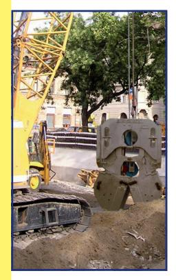
The cutting edges of the grab jaws are made of Hardox steel 450 and were especially hardened. Easy mounting of the grab jaws for excavation widths 800/1000/1200/1500 mm. All the grab teeth as well as all the wire rope pulleys are quickly exchangeable due to their construction as ready to use components.
