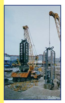
The cutting edges of the grab jaws are made of Hardox steel 450 and were especially hardened. Easy mounting of the grab jaws for excavation widths 800/1000/1200 mm. All the grab teeth as well as all the wire rope pulleys are quickly exchangeable due to their construction as ready to use components.
