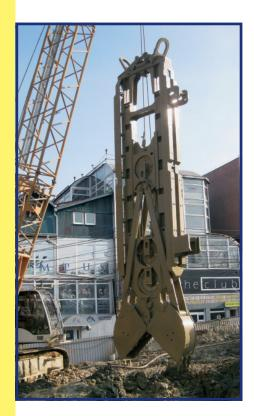
The cutting edges of the grab jaws are made of Hardox steel 450 and were especially hardened. Easy mounting of the grab jaws for excavation widths 600/800/1000 mm. All the grab teeth as well as all the wire rope pulleys are quickly exchangeable due to their construction as ready to use components.
