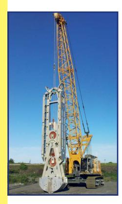
The cutting edges of the grab jaws are made of Hardox steel 450 and were especially hardened. Easy mounting of the grab jaws for excavation widths 1000/1200/1500mm. All the grab teeth as well as all the wire rope pulleys are quickly exchangeable due to their construction as ready to use components.
